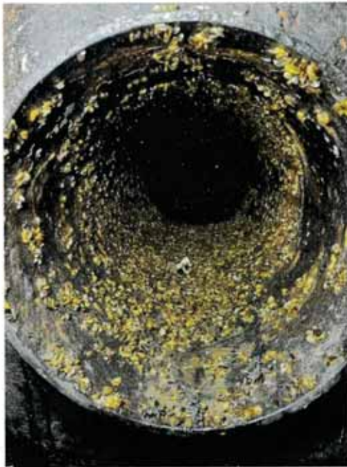
Golden mussels colonizing the inside of a water pipe. SOURCE: Presentation by Arvin-Edison Water Storage District
