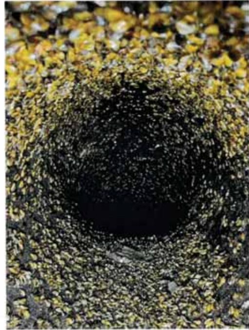
Golden mussels colonizing the inside of a water pipe. SOURCE: Presentation by Arvin-Edison Water Storage District
